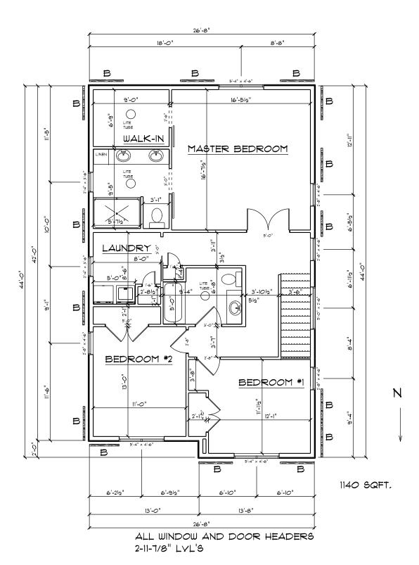
B - 48" BRACE WALL PANELS ALL EXT, SIP WALLS ARE CONTINUOUS OSB SHEATHING, WIND CAT, C 2ND FLOOR PLAN
