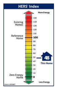
Home Type: Single family detached "Perks" Residence Community: N/A Conditioned Floor Area: 2,173 sq. ft. Number of Bedrooms: Primary Heating System: Ground Source Heat Pump • Electric • 4.8 COP Primary Cooling System: Ground Source Heat Pump • Electric • 24.1 EER Primary Water Heating: Water Heater • Electric • 0.93 Energy Factor House Tightness: 471 CFM50 (0.83 ACH50) Ventilation: 70.0 CFM • 50.0 Watts Duct Leakage to Outside: 57 CFM25 (2.62 / 100 s.f.)
