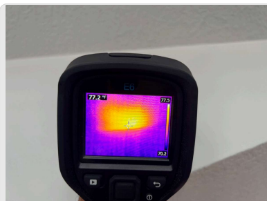
Possible air infiltration (or missing insulation) at soffit above front entry door. Note soffit is within conditioned space.
