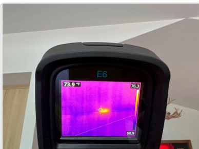
Possible air infiltration (or missing insulation) at soffit above front entry door. Note soffit is within conditioned space.
