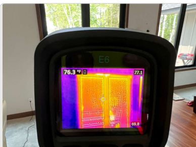
Possible air infiltration (or missing insulation) at soffit above front entry door. Note soffit is within conditioned space.
