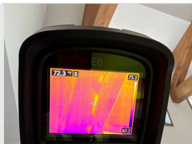
Possible air infiltration (or missing insulation) at soffit above front entry door. Note soffit is within conditioned space.
