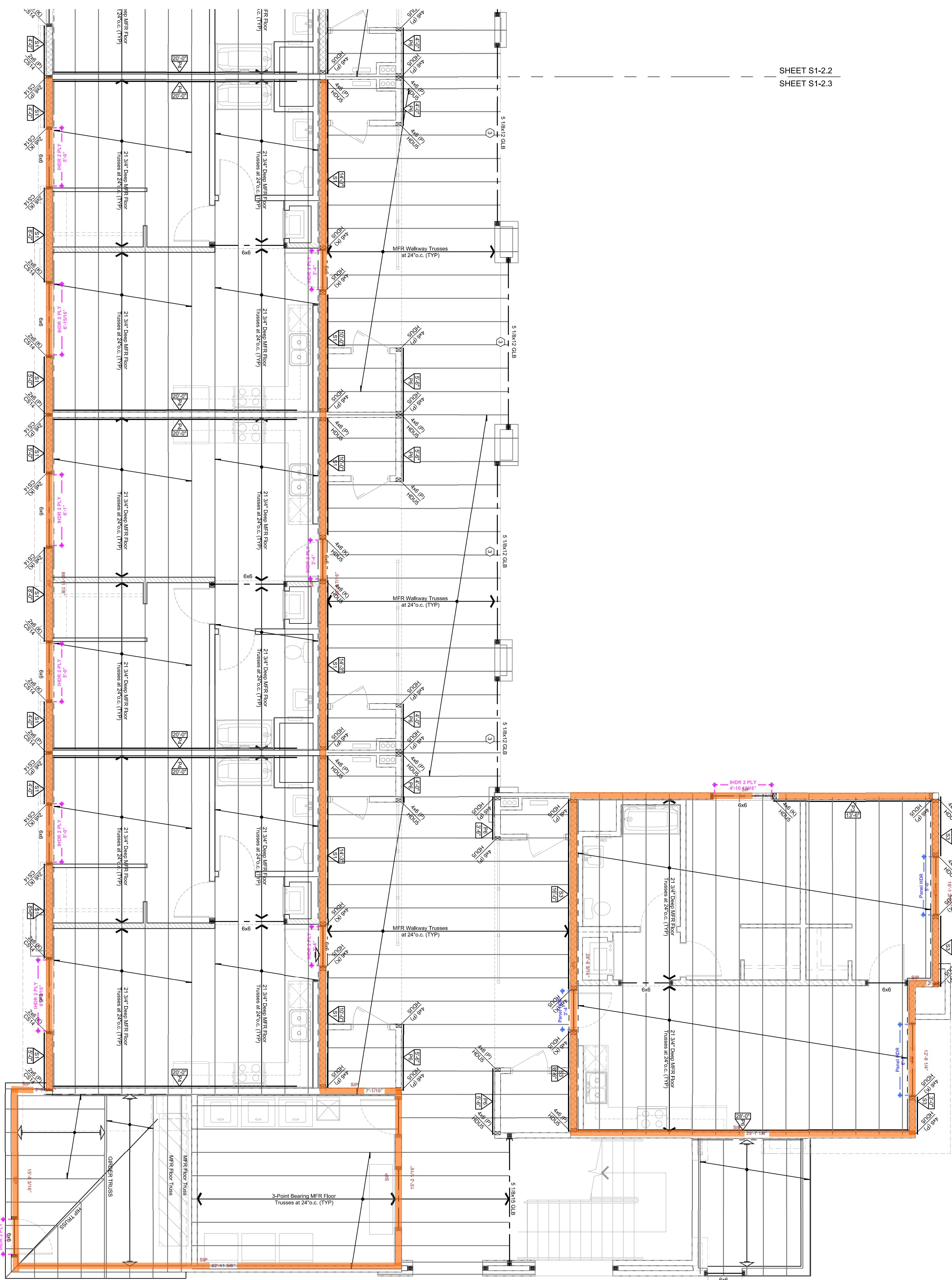
ENLARGED 1st FLOOR FRAMING PLAN
